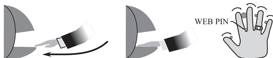
Figure 8-2: Placing Your Hand on the Platen
